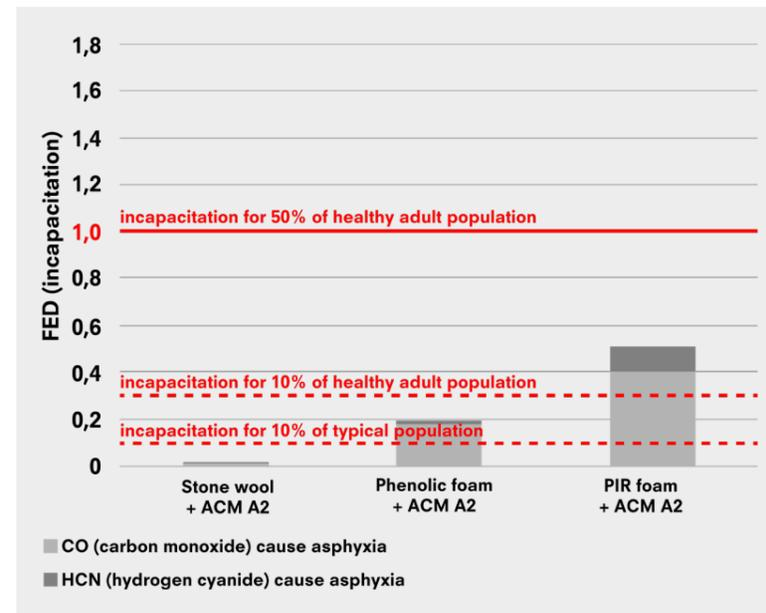
Contribution of CO, HCN, CO<sub>2</sub> and lack of O<sub>2</sub> to lethality (ISO 13344) at 30 minutes for gases entering a 50m<sup>3</sup> room from cladding through 100mm vent:
