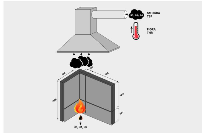
The classification parameters of the SBI test are fire growth rate index (FIGRA), lateral flame spread (LFS), and total heat release (THR600s). Additional classification parameters are defined for smoke production as smoke growth rate index (SMOGRA) and total smoke production (TSP600s), and for flaming droplets and particles according to their occurrence during the first 600 seconds of the test.
